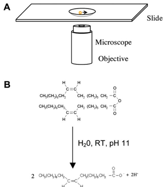
**Figure 1.** Experimental setup. (A) The concave depression in the glass slide was filled with 100  $\mu\text{L}$  of aqueous solution. A small drop of oil was added by pipet and observed with an inverted microscope. (B) Oleic anhydride was hydrolyzed in the presence of water at high pH and room temperature to form two amphiphiles. Note that at high pH the fatty acids were deprotonated.
