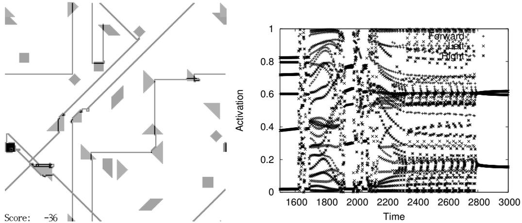
Figure 4. An example of movement of the same agent in another environment. The wandering phase takes longer than for the former example. In the latter period of the wandering phase the agent moves obliquely. After encountering a square object, its movement changes to the examining phase, but accidentally leaves the object. It happens to reenter the object and succeeds in switching to the filling phase. The memory of touching a candidate square is retained.
