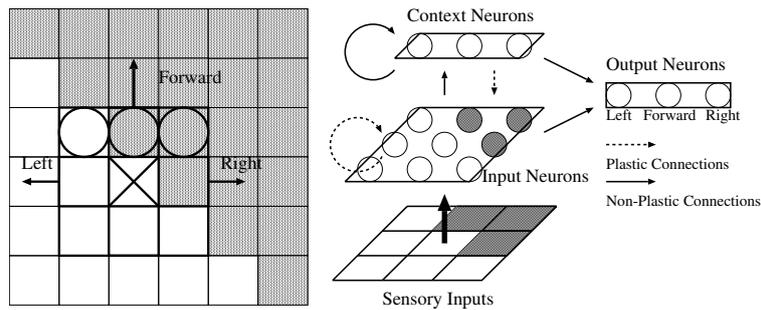
Figure 1. An agent with neural network architecture is situated in the environment. The architecture consists of nine sensory inputs that are connected to corresponding input neurons. Three context neurons are used to keep short-term memory in unit cubic space. Movements are decided by the most activated neuron of the three output neurons related to moving forward, left or right. Connections to input neurons are plastic and updated according to the sensory inputs.
