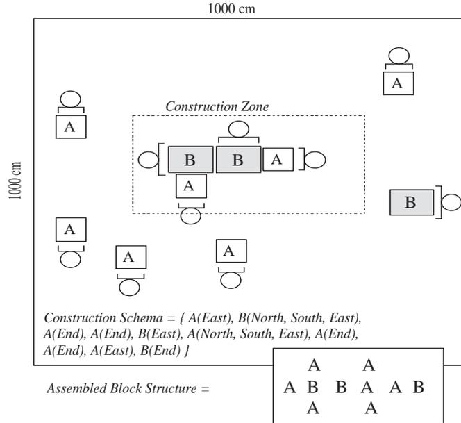
Figure 3: *Gathering and Collective Construction (GACC) Example*. Seven type A, and three type B blocks are randomly distributed throughout the environment. In the construction zone, five blocks are connected as a partially assembled structure. The construction schema and target structure are given at the bottom. The team uses 10 robots.
