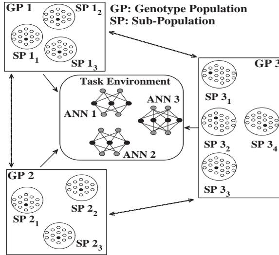
Figure 1: *CONE Example*. A controller is evolved in each population. All controllers are evaluated in a collective behavior task. Double ended arrows indicate self regulating recombination occurring between populations. ANN: Artificial Neural Network (controller). GP X: Genotype Population X. SP X<sub>z</sub>: Sub-Population z in Genotype Population X.
