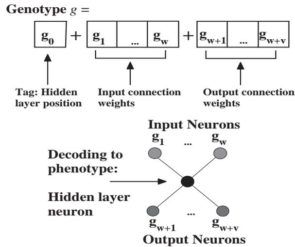
Figure 2: *CONE Genotype*. There is a direct mapping between a genotype and a hidden layer neuron. A genotype has  $w$  genes indicating the neuron's input connection weights, and  $v$  genes for the neuron's output weights. A tag ( $g_0$ ) specifies the neuron's position in a controller's hidden layer, and hence the sub-population to which the genotype belongs.
