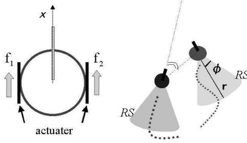
Figure 1: Left: a schematic view of the mobile robot with two wheels (actuators). It computes the forward force vector and the torque strength from the force vector  $(f_1, f_2)$  on each actuator. Right: Two mobile robots interact to perform turn-taking behaviour by sensing each other’s position, relative distance and heading angle. It is robot A’s turn when A enters the area that is B’s rear side (RS) position. The shape of this RS is parameterized by  $r$  and  $\phi$ .
