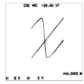
Figure 1 (Aihara & Ryeu). A return plot of a chaotic neuron electronically implemented with an analog electronic circuit.
