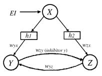
Figure 3 (Aihara & Ryeu). A chaos-driven contracting system with external input EI to the chaotic neuron X and Heaviside transfer functions  $h_1$  and  $h_2$  from the chaotic neuron X to the static neurons Y and Z.
