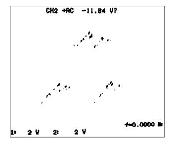
Figure 2 (Aihara & Ryeu). Fractal-like structure observed on the Y-Z space in an analog electronic circuit of a chaos-driven contracting system of Figure 3.
