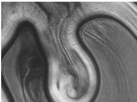
Figure 1 The hydrolysis of the oleic anhydride oil (top and centre) in the presence of alkaline water
